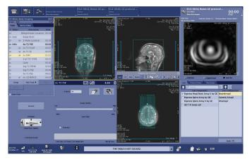
The Slider Bar is designed to help you select optimal scan-time for the most routine exam protocols by selecting within the recommended 5 levels of scantime-resolution combinations. The parameters behind each level are optimized, such that even with the recommended shortest scan-time, the fundamental contrast
